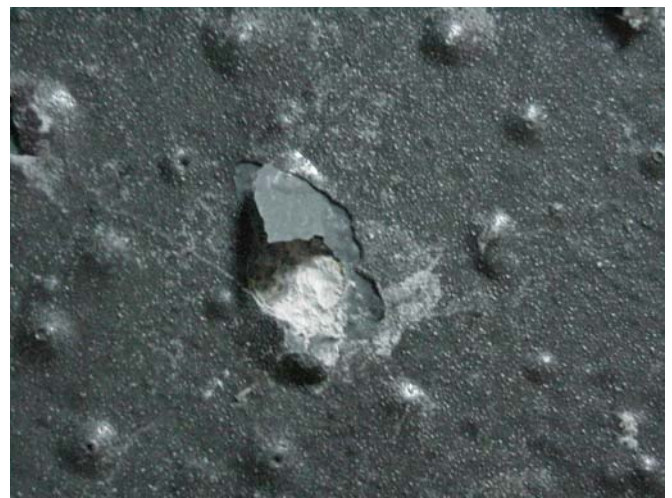
Figure 9: substrate “volcanoeing” at pinhole
