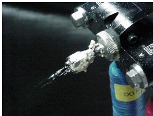
Figure 6: Plugged air purge spray gun; moving mixing chamber / valving rod
